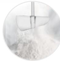
**The Rapid Visco Analyzer™** measures performance of ingredients. Test the binding and texture enhancing characteristics of starches, binders, gels, and stabilizers used in meat products. Verify all incoming materials meet performance specifications before they enter production. This helps reduce line shut downs, re-work, scrap, and optimize their use.
