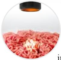
**The DA 7440** is installed over conveyor belts and measures fat, moisture and protein of meat products. Measure coarsely ground raw meats or in-process samples. The instrument continuously measures and stores results which can then be used to characterize and summarize an entire batch. Use the measurements to reduce fluctuations in fat in real-time and improve end product quality.
